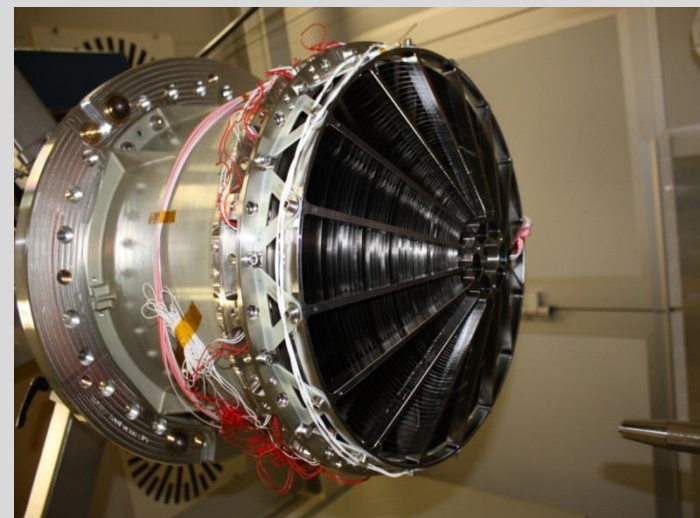
eROSITA 7 \times 54 mirror shells
