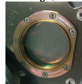
Filter mounted on support structure
