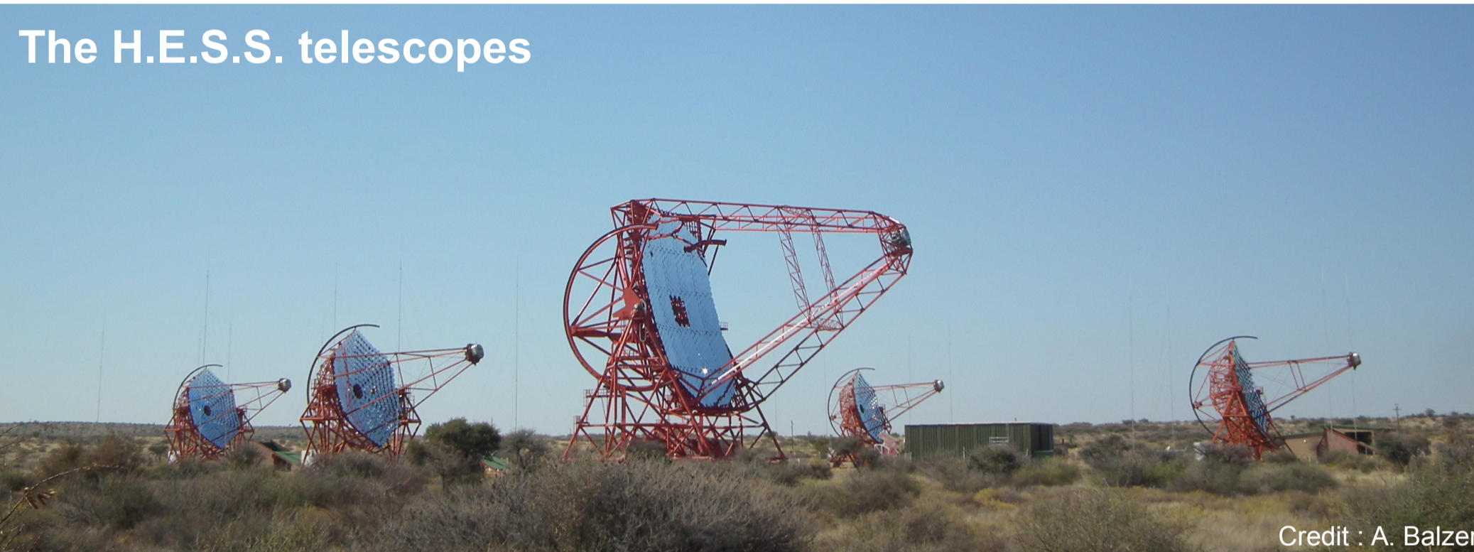
FIG. 1 : The H.E.S.S. Telescopes. Located in Namibia, this array of Imaging Atmospheric Cherenkov Telescopes detects very-high energy gamma rays. In its first phase (2004 – 2012), the array had 4 telescopes. The fifth, largest, telescope was added in July 2012. The analysis presented here uses only data taken with the original array.
