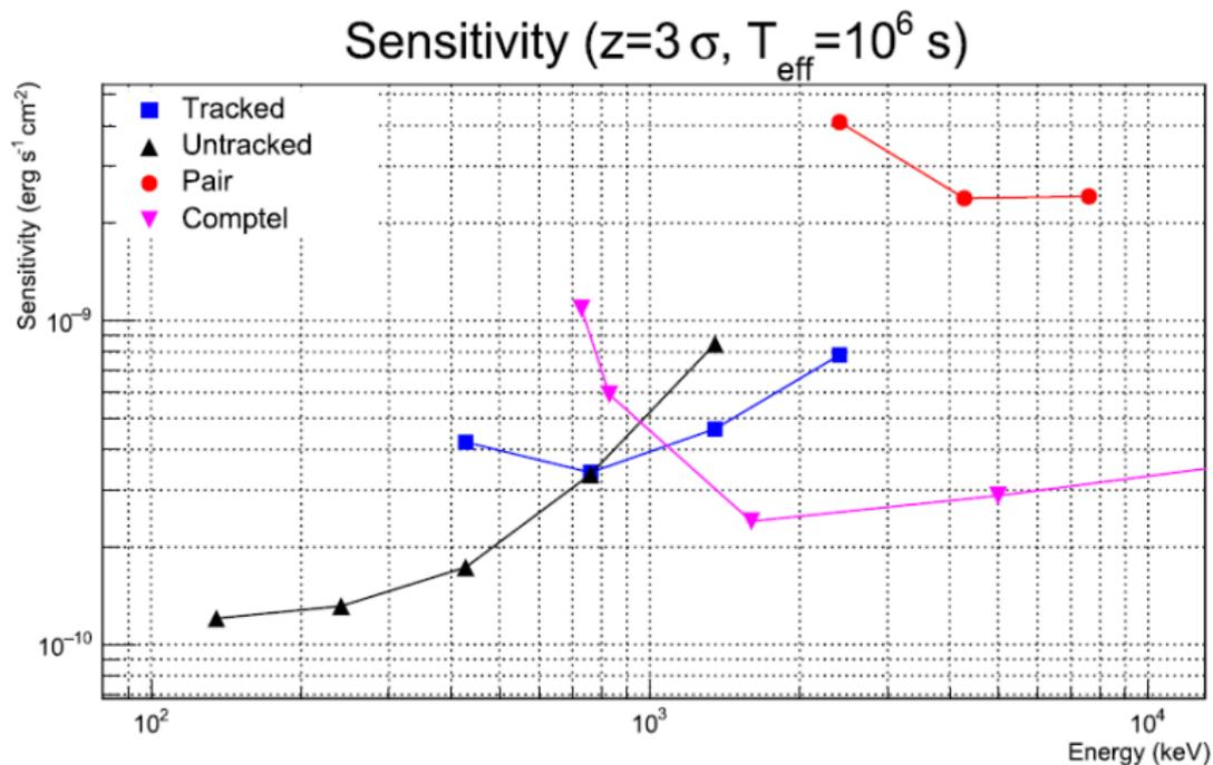
Fig: sensitivity for the detector compared to COMPTEL's (no activation background).
