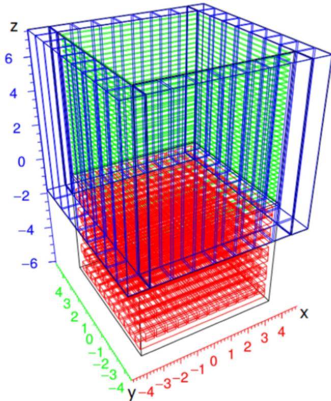
Fig: a schematic of the detector (no anticoincidence shield).
