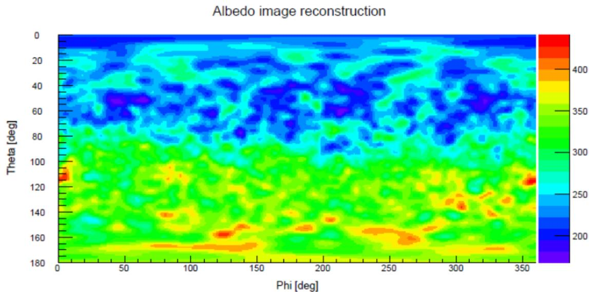
Fig: Albedo reconstruction with the detector pointing normally outwards the Earth.
