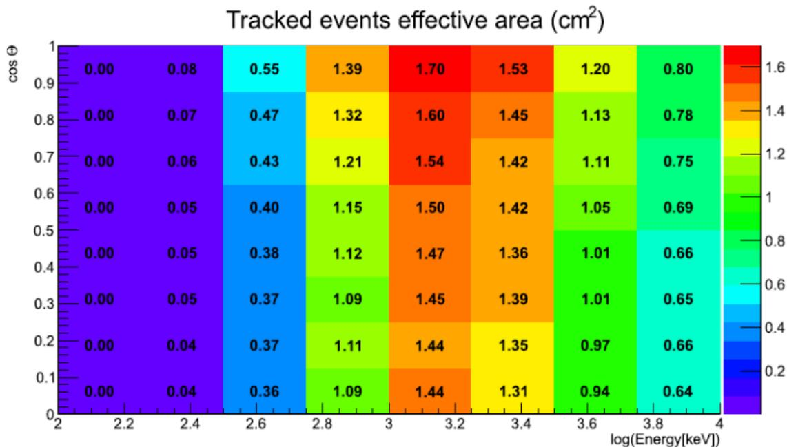
Fig: effective area for tracked events as function of incident photon energy and angle.
