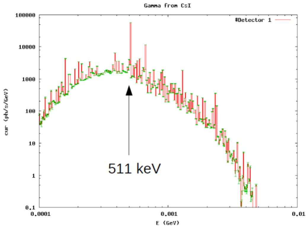
Fig: gamma photons exiting the calorimeter due to activation.
