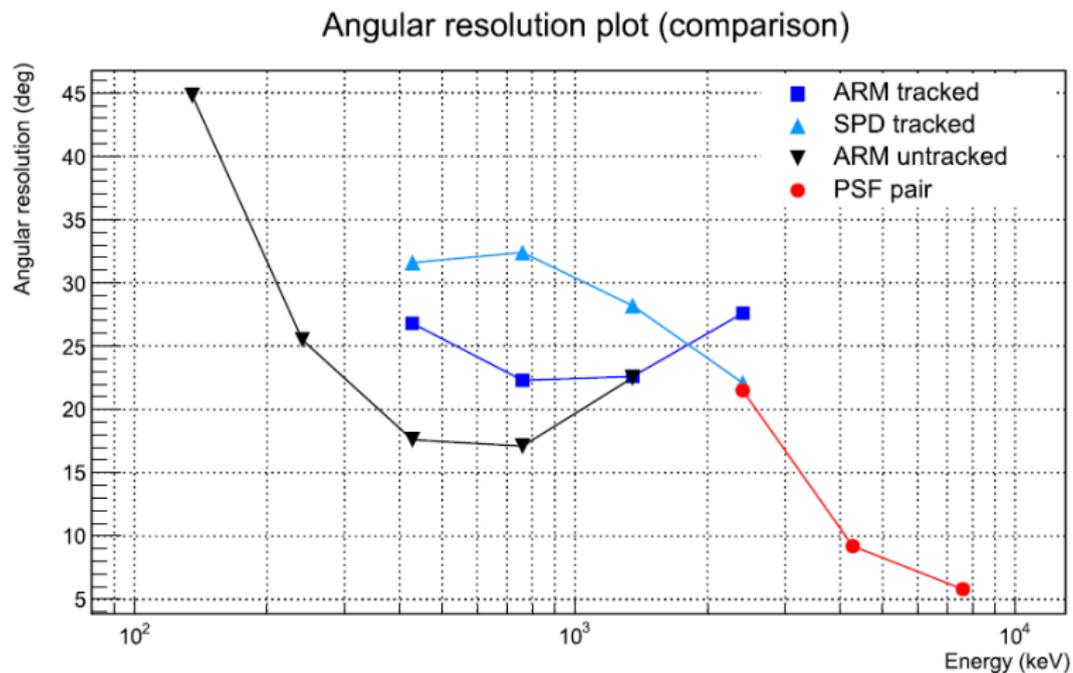
Fig: angular resolution for different types of events.
