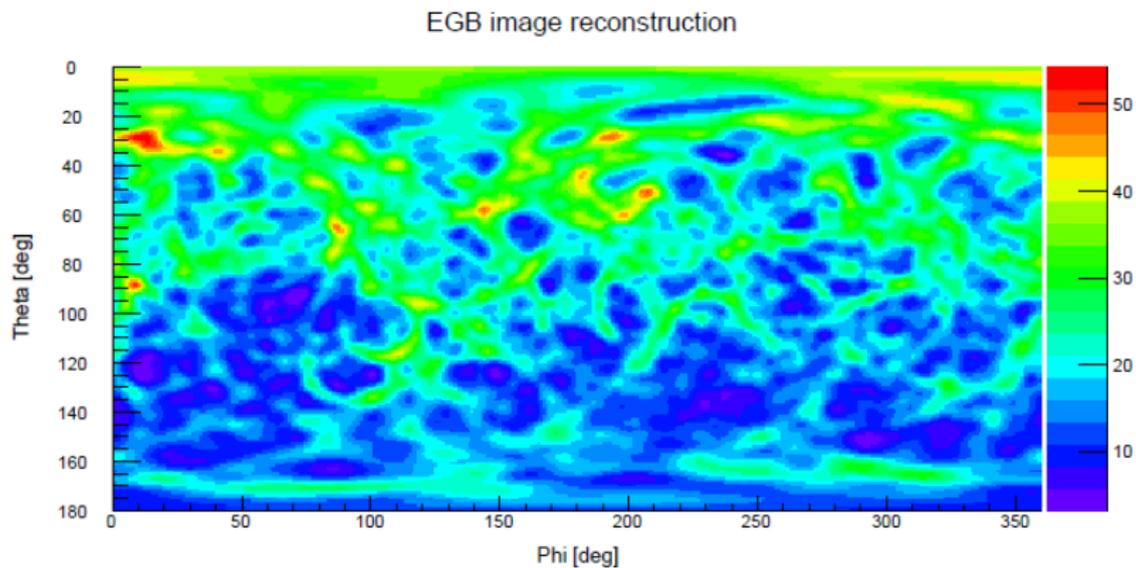
Fig: EGB reconstruction with the detector pointing normally outwards the Earth.
