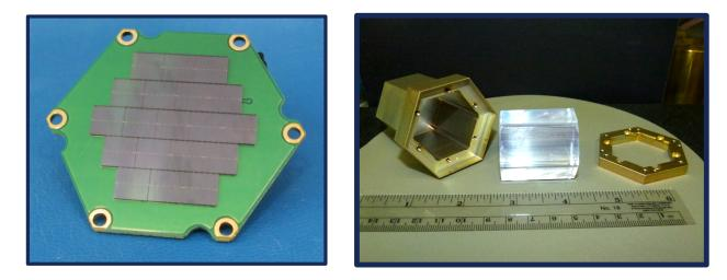
SrI2:Eu detectors developed for use on SIRI-2. MERGR detectors would be identical, expect for thickness. (Top) Exploded CAD rendering of detector assembly. (Bottom left) 19-element SiPM array developed by NRL for read out of hexagonal crystals. (Bottom right) SIRI-2 flight model hexagonal crystal prior to installation into detector housing.
