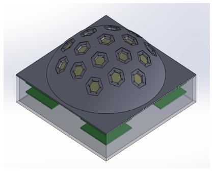
Right: CAD rendering of MERGR from the instrument's zenith showing the locations of the 19 hexagonal detectors in a closelypacked dome geometry.
