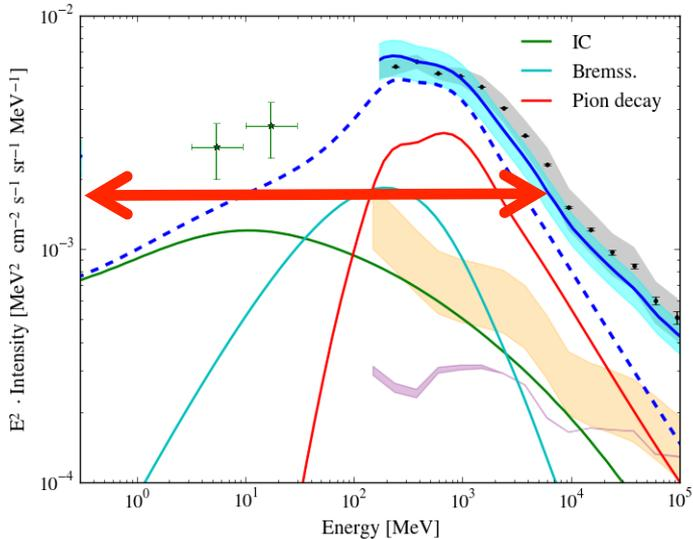
Predictions for the energy range of e-ASTROGAM and AMEGO, possible future gamma-ray instruments for model R, as an example. The figure shows also the Fermi LAT data intermediate latitudes [1] and COMPTEL data [9] for comparison.
