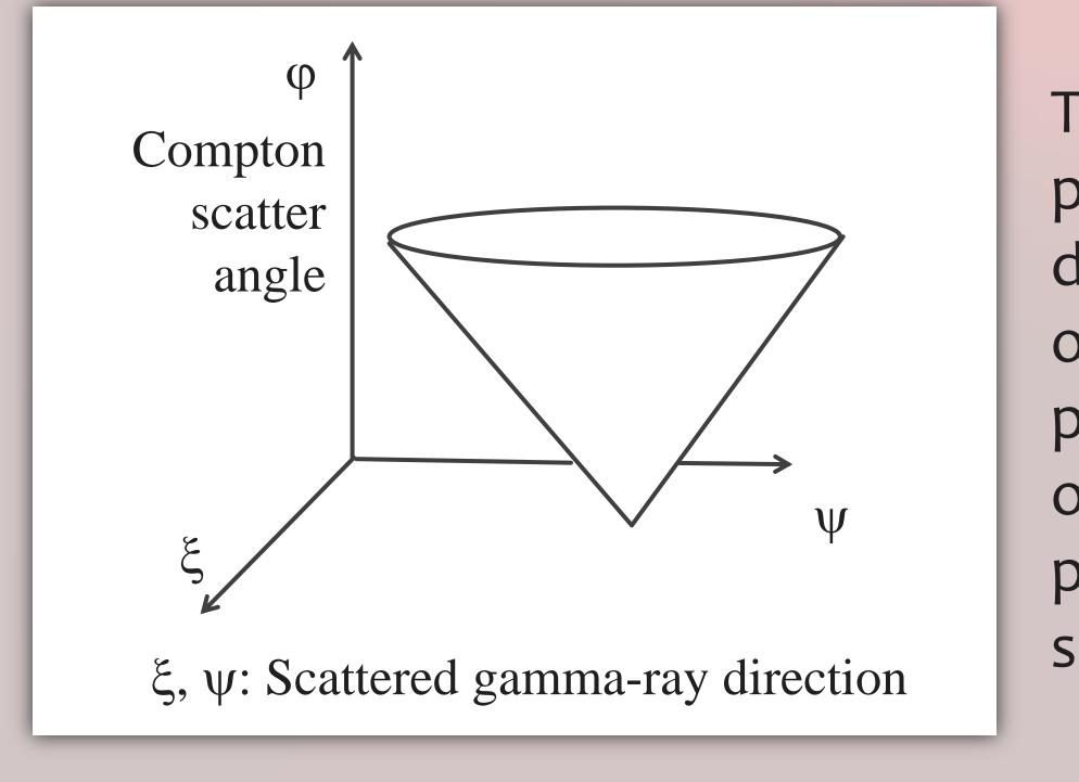
The point spread function of a point source in the COMPTEL data space is a cone with an opening angle of 90 degrees pointing at the direction of origin of the gamma rays in the plane of the direction of the scattered gamma ray.
