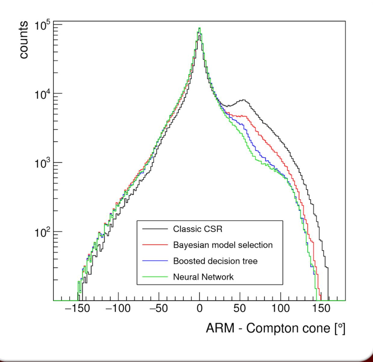
Comparison of different Compton event reconstruction approaches using COSI's 511-keV calibration data: The narrowest (ARM) distribution shows the best event reconstruction approach (here: neural network).
